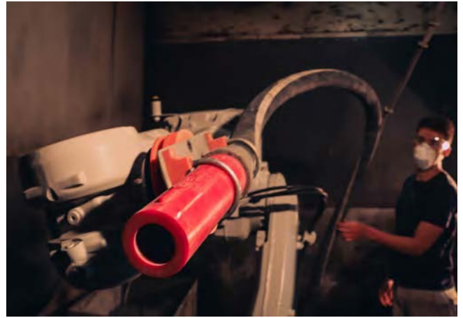
Robotic arm with shotcrete nozzle in the lab
