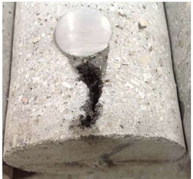
Fig. 2: This core specimen's major flaw is evidence of inadequate flow during placement.
